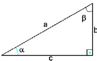
$$\text{sen } \alpha = \frac{b}{a} \quad \text{cos } \alpha = \frac{c}{a} \quad \text{tg } \alpha = \frac{b}{c}$$
